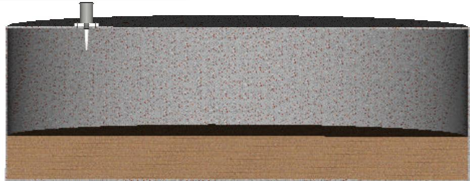
Application History: These customers tried several ultrasonic level detectors that didn't work because of methane. Some radar units were also used, they had echo stability problems which gave false readings.
