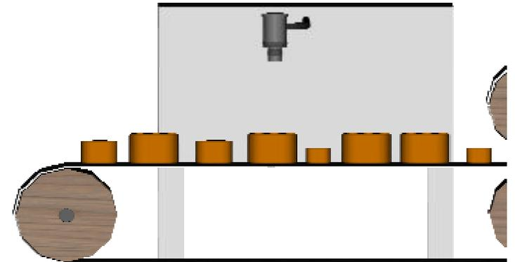
Application Problems: Very narrow tanks with welding joints on the walls, close mounting of the ultrasonic device to the wall (12inch). Material in tanks is gravel mixed with sand.
