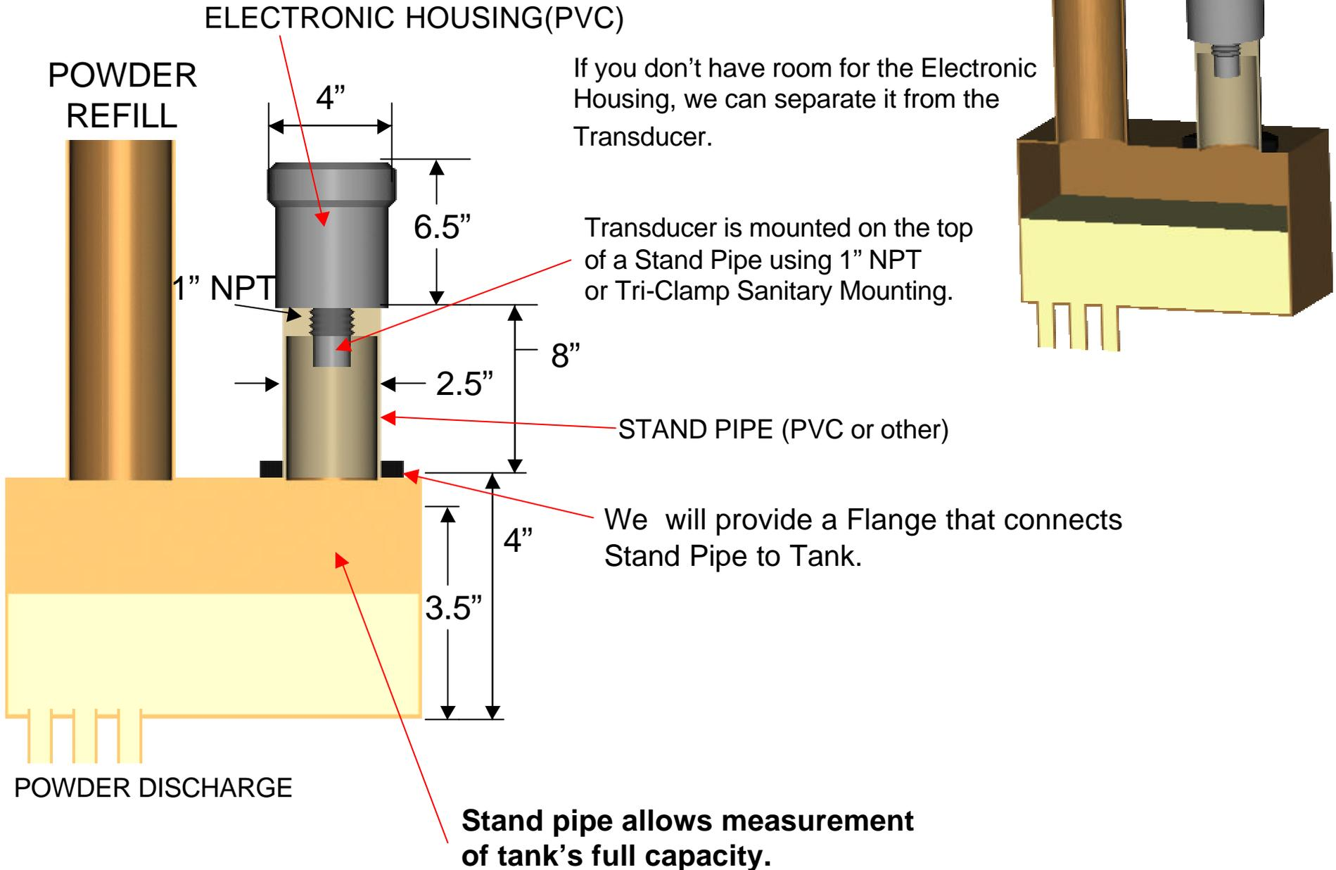
Application Problems: To measure level of liquids in pipe attached to a tank.
