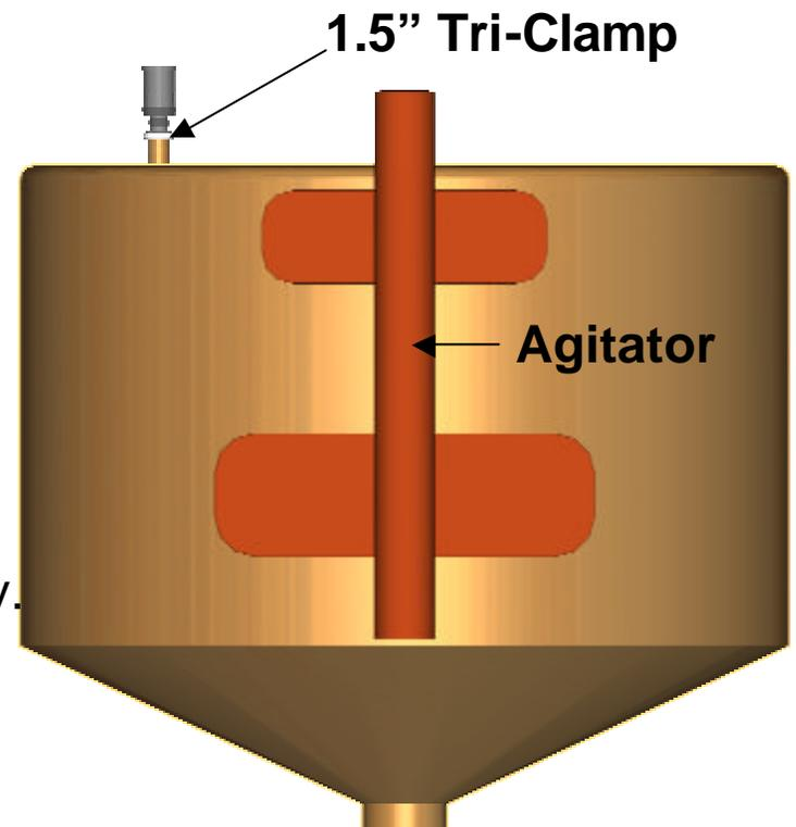
Application Problems: Metal tank consists of Sulfuric Acid with a strong vapor. Mounting hole is only 10" away from tank's wall, and there is a standpipe of 3" ID and 6" long.
